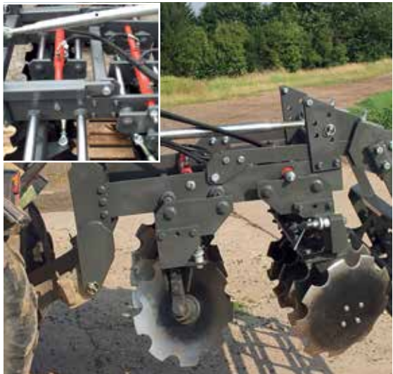
Disc harrow (width adjustment)
