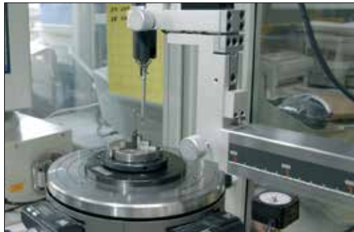
Measuring the inner diameter of a press-fitted bearing
