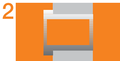
Assembly of iglide® bearing with transition fit
